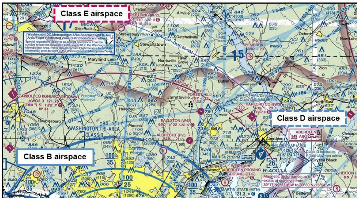
Figure 1-1-4: Aeronautical Chart with Airspace Classifications
